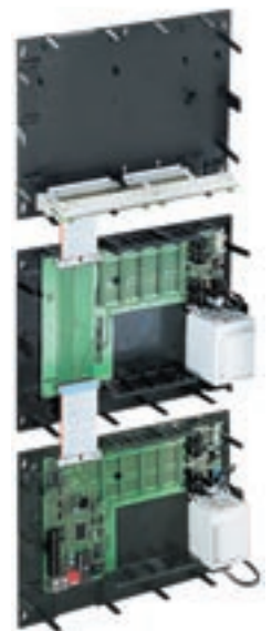
Basic Central (bottom) with Expansion Housing (center) and Interface Housing (top).
